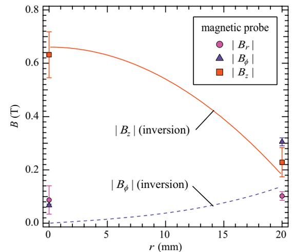
FIG. 6. Determined radial profiles of the magnetic field strengths. The dashed line represents  $|B_\phi|$  and the line represents  $|B_z|$ . Markers: the filled circles, triangles, and squares, respectively, represent the  $r$ -,  $\phi$ -, and  $z$ -components of the magnetic probe data (#12758).
