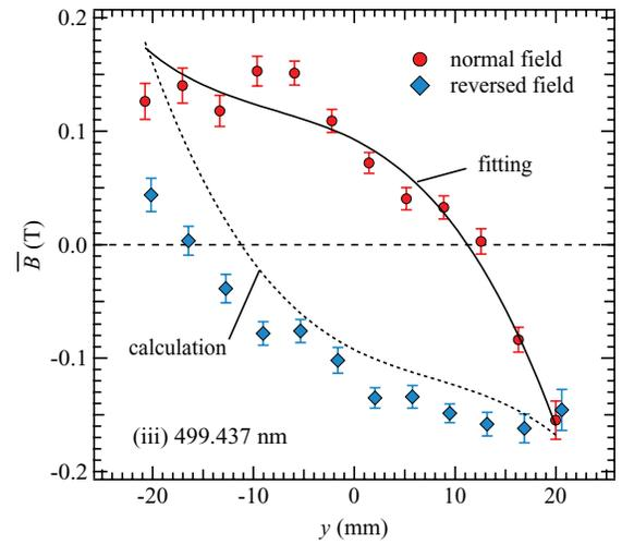
FIG. 5. Measured “apparent” magnetic strengths from spectral line (iii) with the normal (#12970) and reversed (#13008) poloidal field directions. The line denotes the fitting result to the normal field data. The dashed line denotes the field-strength expected to be observed in a reversed field discharge; it is calculated by using the determined  $B_\phi$  and  $B_z$  profiles in the normal field discharge plotted in Figure 6.
