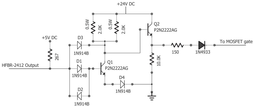
Fig. 3. Circuit for triggering the MOSFET switch.
