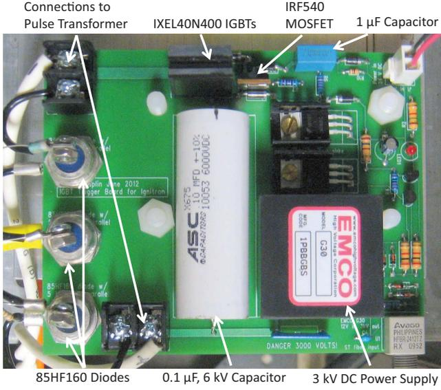
Fig. 4. Photo of finished ignitron trigger board. The board dimensions are 4 inches by 5 inches.
