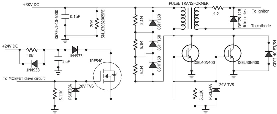
Fig. 2. Partial circuit diagram for the ignitron driver.
