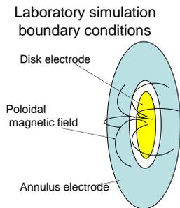
Figure 2. A capacitor bank connected between the central disk and the annulus creates a radial electric field  $E_r$ , which drives current nearly along the poloidal field lines in analogy to the astrophysical situation.
